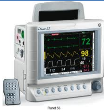
Multi-para monitor with ETCO2 monitor-very useful for monitoring of all types of major and complicated surgeries.
