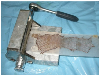
Skin graft Mesher-Apex India-Usefull machine for meshing and expansion of graft for major burns cases.
