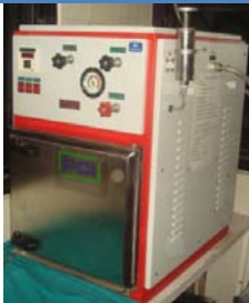
ETO machin- best machine for sterilization of surgery instruments and other articles. First machine in Plastic surgery set up in Maharashtra
